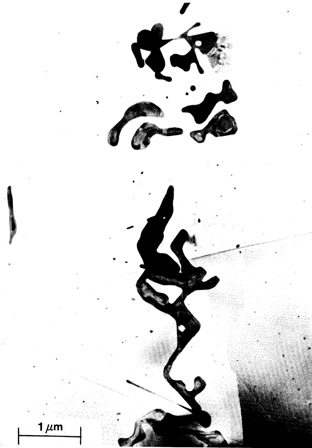
FIG. 3. TEM micrograph of carbon deposited on the basal plane of MoS 2 crystal from exposure to 0.6 atm CH 4 at 700°C for 3 h.
