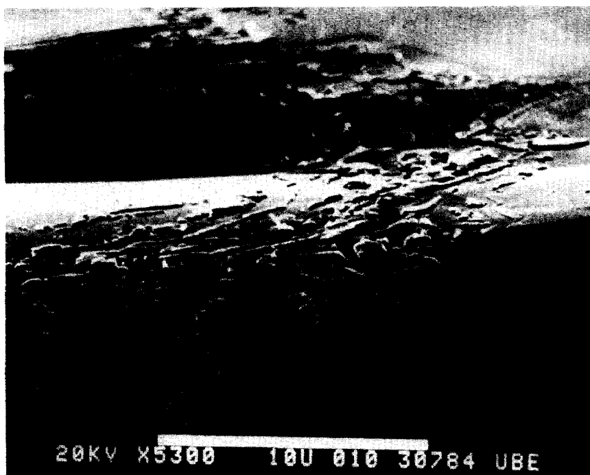
FIG. 4. SEM micrograph of carbon islands formed on the basal plane of \text{MoS}_2 after exposure of the crystal to 0.6 atm \text{CH}_4 at 700^\circ\text{C} for 3 h. Carbon is deposited on the exposure face.
